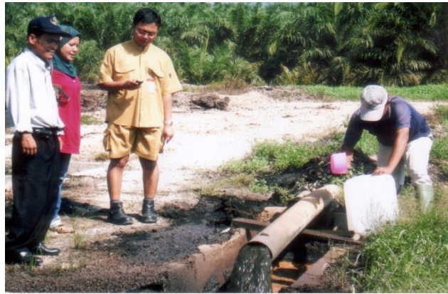
Fig. 6. Waste of CPO in pipe was flowed to sedimentation reservoir throw to gutter.
